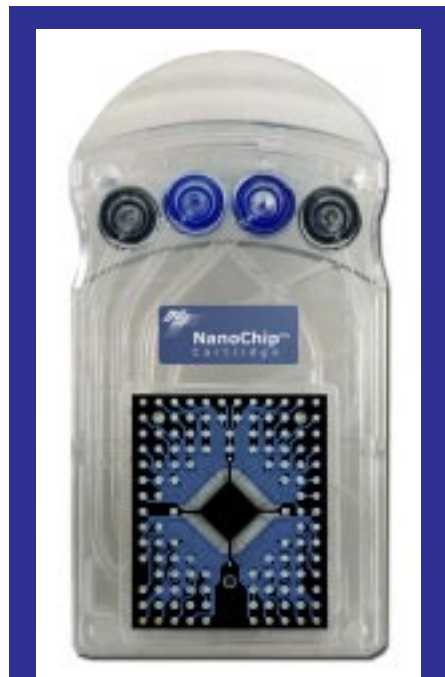
Nanogen's NanoChip™ handheld DNA chip and sample handler; the sample ports are at the top, and the chip is the diamond in the centre.
